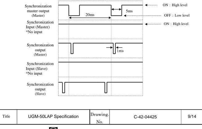
• When the synchronization master output of the master is connected to the synchronization input of the slave, the master sensor can synchronize falling edges of the synchronization master output signal with falling edges of the synchronization output signal.
